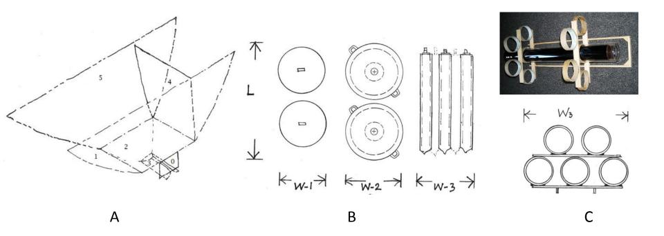
A **thru-wall solar kitchen building** or trailer has a vertical oven door (0 in Fig A); and reflector parts (Fig A): 1 is a reflector wall above the oven door; 2 is a box with horizontal or inclined inlet aperture (unglazed or glazed); 3 is a ridged-pyramid base/bracket; 4 is an E and W end adjustable or repositioned at noon; and 5 is the other side of a two-sided trough.
