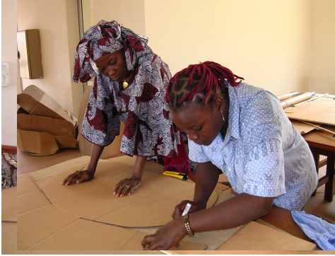
Draw the precise form of the CookIt using a mould
