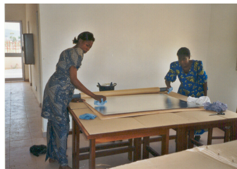
Gently wipe the surface of alum foil with clean and soft cloth
