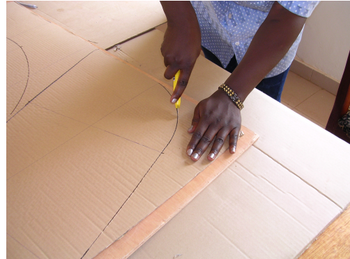
Mark all the fold lines and points using the mould, (CookIt example)
