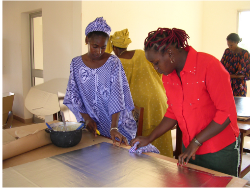
Repairing gluing after quality control
