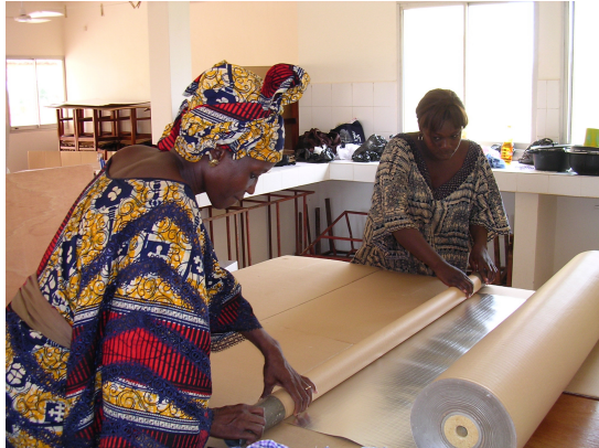
Transferring aluminium from the heavy, big roll onto small rolls
