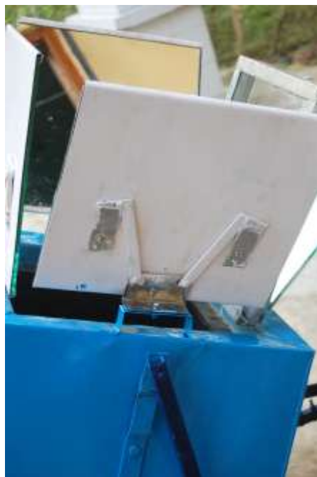
PHOTOGRAPH.4- Shows the close-up view of reflector holding system
