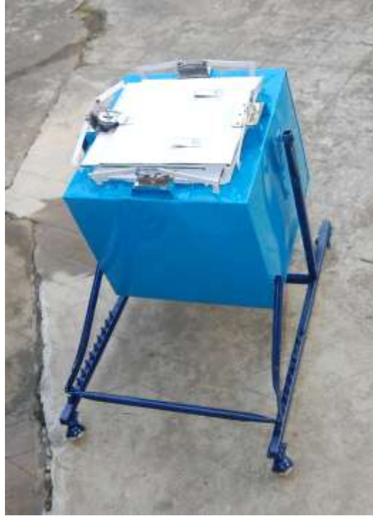
PHOTOGRAPH.5- Shows the reflectors in folding position
