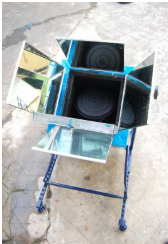
PHOTOGRAPH.2- Shows the cooking pot inside of oven
