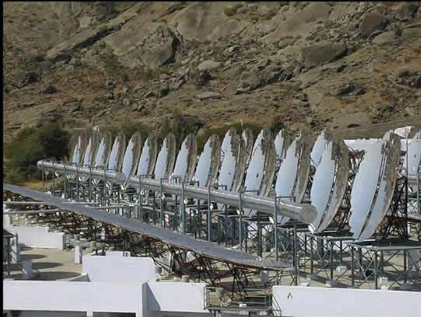
Large-scale, Scheffler, roof-top parabolic solar cooker system in India
