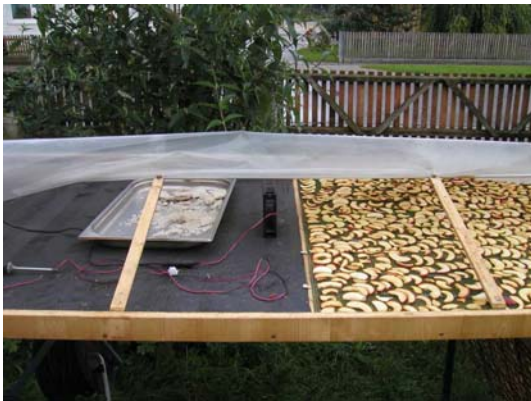
Dryer with tray with Calcium Chloride, fan and apples
