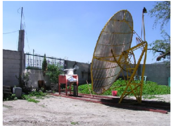
Picture 9: testing the 8m 2 Scheffler Reflector
