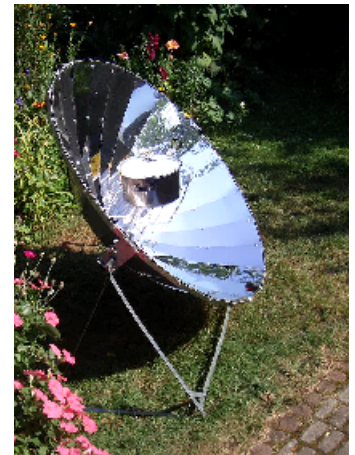
Fig. 2 Test result of solar concentrator cooker K14 on 1 October 2002 at latitude 48°N (6)
