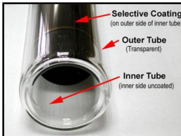
Figure 3. Construction of a Al/N/Al coated evacuated tube.
