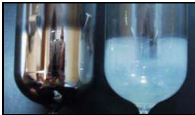
Figure 5. The appearance of the barium getter layer in a tube with a good vacuum at the left and the appearance of it in a tube with no vacuum at the right.
